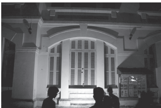
Fluorescent 18W – floodlighting
