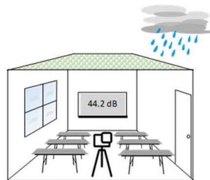
Raining with green roof
