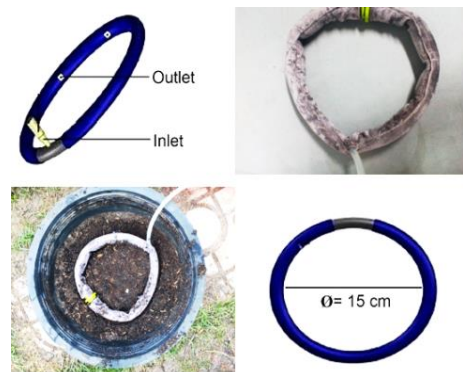
Figure 6 The developed ring-shaped emitter based on Kansei Engineering.
