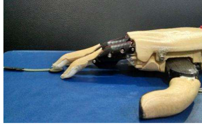
Figure 19 Grip force measurement using the FSR sensor.
