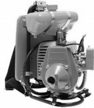
Figure 9 Petrol engine used as power source in the power weeder (Model-BG-328, Brand-SAIMAC, Country-China).
