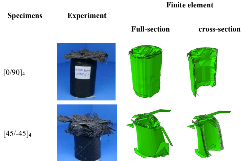
Figure 3 A comparison of the damage behavior of carbon tubes upon impact in the experiment and FEA model.
