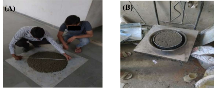
Figure 1 (A) Slump flow and (B) sieve segregation tests for SCC.
