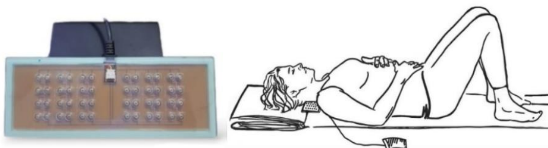
Figure 2 LLLT pad (48 LED diodes, wavelength 660 nm; PRIMA Laser therapy, Thailand) and its application to the trapezius muscle.
