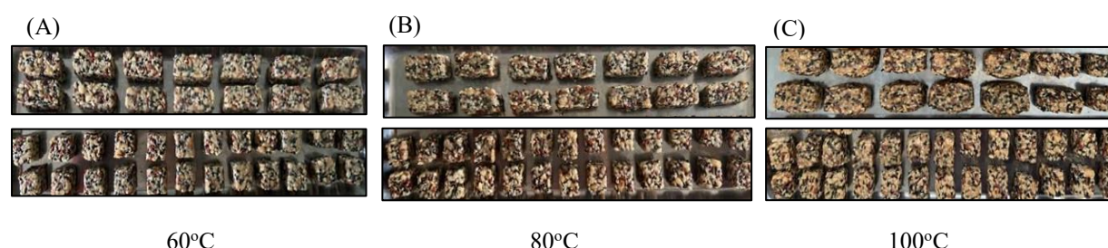
Figure 5 Krayasart bars after being dried at (A) 60°C, (B) 80°C, and (C) 100°C.
