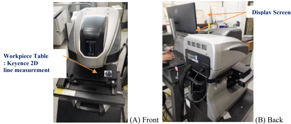
Figure 4 Displaying the surface measurement using Keyence 2D line measurement (non-contact/vision).
