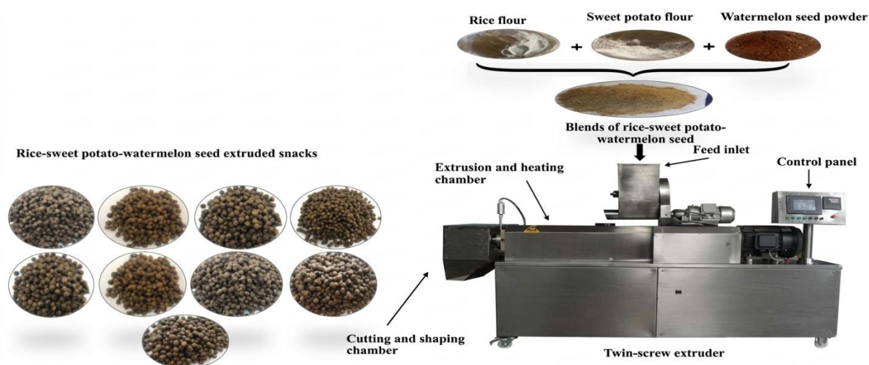
Figure 1 Schematic of the extrusion process for rice–sweet potato–watermelon seed blends using a co-rotating twin-screw extruder
