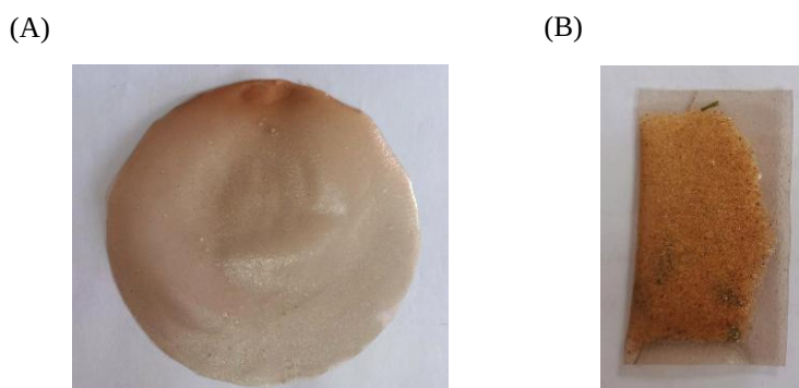
Figure 2 (A) Biofilm and (B) instant noodle seasoning packet prepared from jackfruit seed starch.
