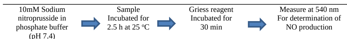
Figure 2 Scheme for NO radical scavenging assay [14]
