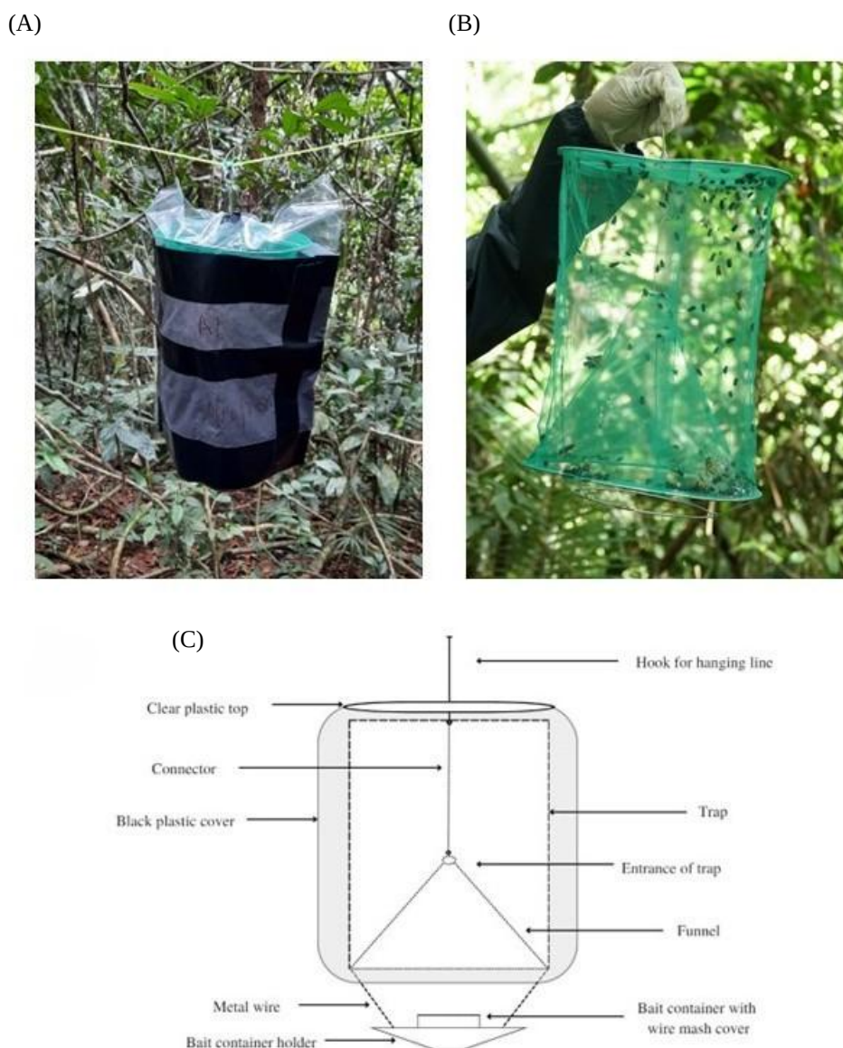
Figure 2 (A) Modified minnow trap suspended and covered with a plastic bag to prevent rain from destroying the sample. (B) A modified minnow trap containing captured blowflies. (C) Schematic diagram of a modified minnow trap.
