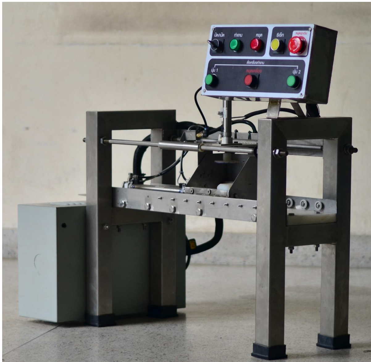
Figure 8 The ready-to-work durian stick processing machine.
