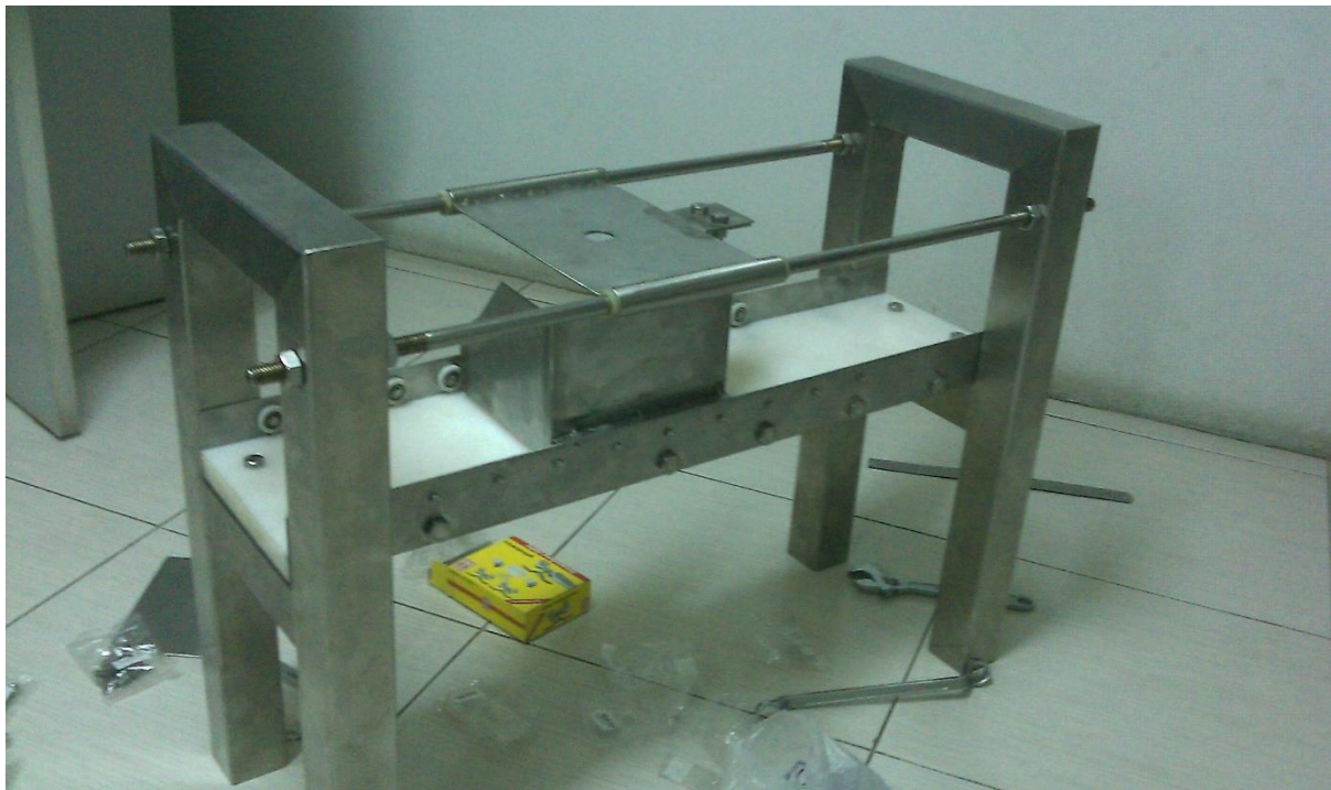
Figure 7 Structure frame of the durian stick processing machine.
