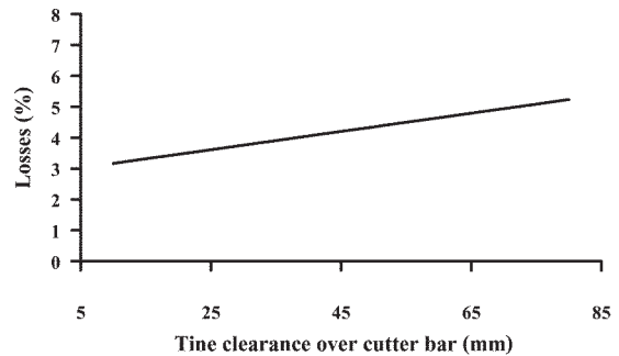
Figure 7. Correlations between tine clearance over cutter bar and losses
