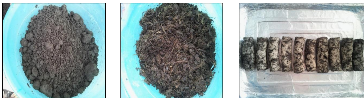
a. Dried wastewater sludge b. Dried banana peel waste c. Briquette-derived fuel Figure 1 Raw materials used in the test and the finished briquette-derived fuel.
