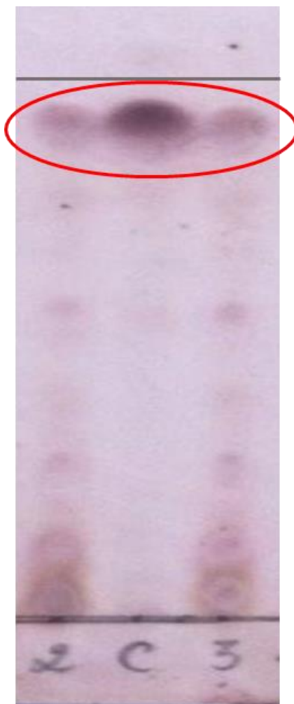
Figure 2 Thin layer chromatography plate of SLs: 2,3: SLs sample, C: SLs standard (1',4''-Sophorolactone 6',6''-diacetate).
