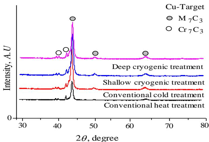
**Figure 4** XRD patterns of treated specimens.
