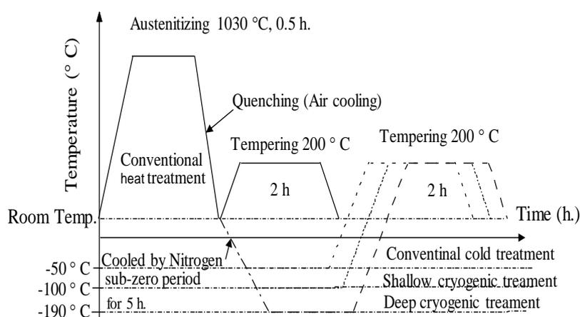
**Figure 1** Treatment processes of SKD 11 specimens in this experiment.
