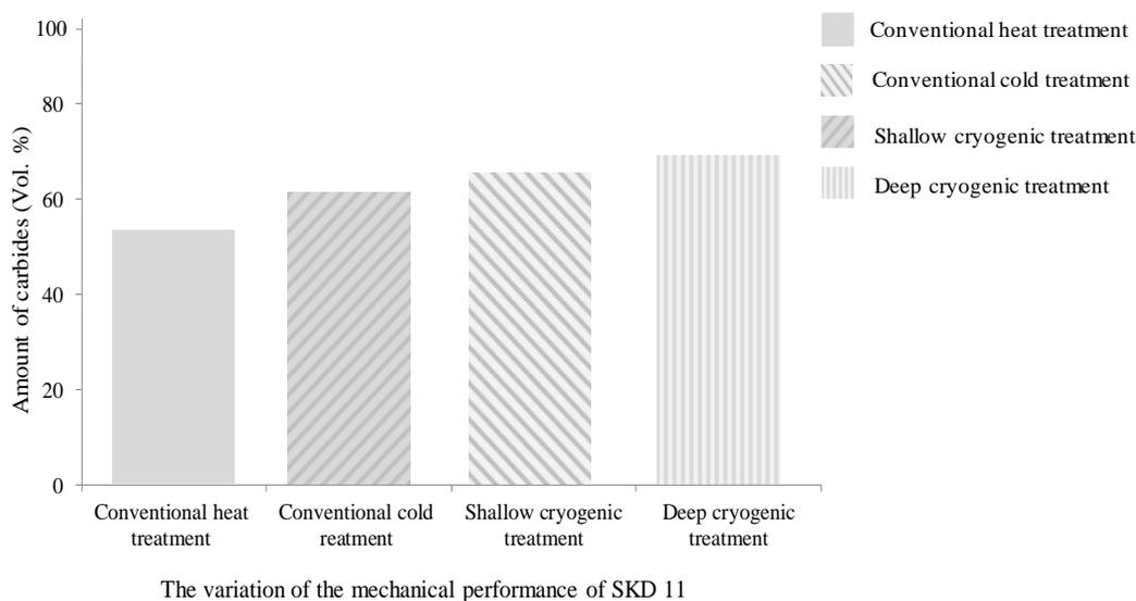
**Figure 5** Estimated amount of carbides of different heat-treated SKD 11 specimens.
