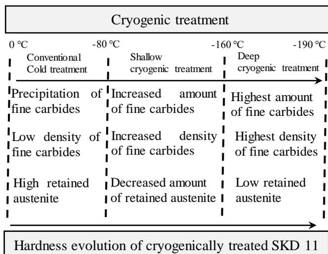
**Figure 7** Schematic diagram illustrating the hardening evolution of SKD 11 tool steel submitted to cryogenic treatment.
