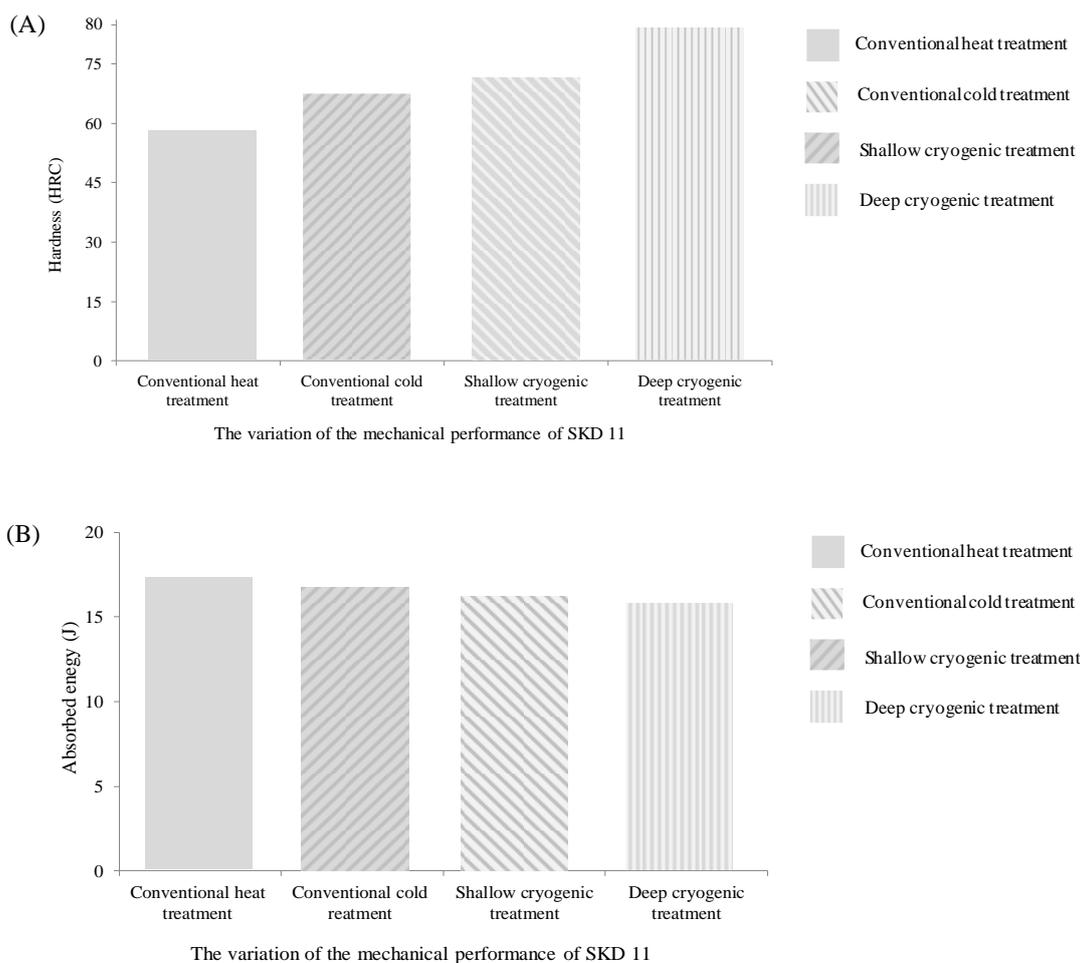
**Figure 6** Mechanical performance of different heat-treated SKD 11 specimens: (A) hardness; and (B) impact toughness.
