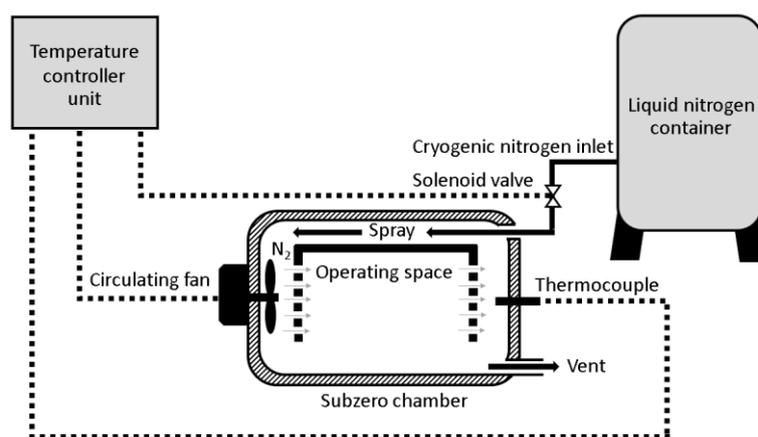
**Figure 2** Schematic diagram of the self-made liquid nitrogen treatment system.
