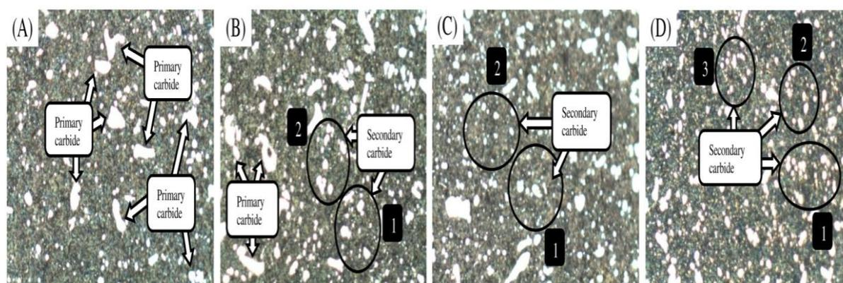
**Figure 3** Micrographs of specimens (at  $50\times$  magnification): (A) Conventional heat treatment; (B) Conventional cold treatment; (C) Shallow cryogenic treatment; and (D) Deep cryogenic treatment.
