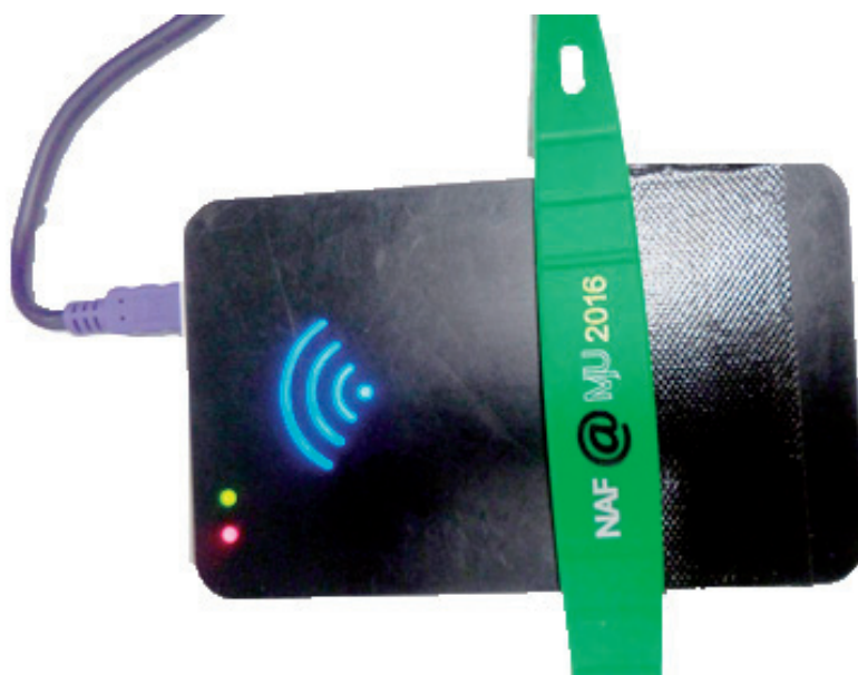
Fig. 11. Write ID into wristband tag by UHF RFID desktop reader.
