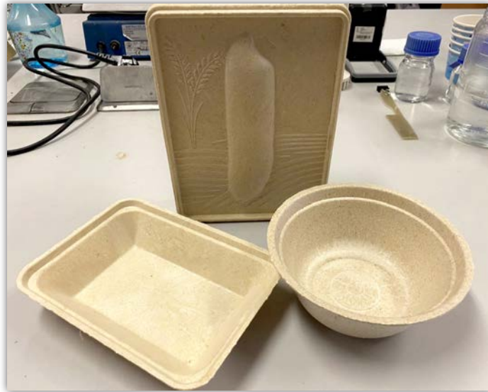
Figure 12 Example of thermoplastic starch products from bamboo waste can be made using semi-compression process
