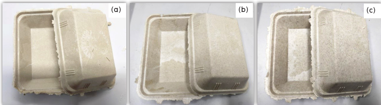
Figure 10 Thermoplastic product prepared from various size of bamboo waste powder; (a) 0.5 mm, (b) 1.0 mm and (c) 2.3 mm
