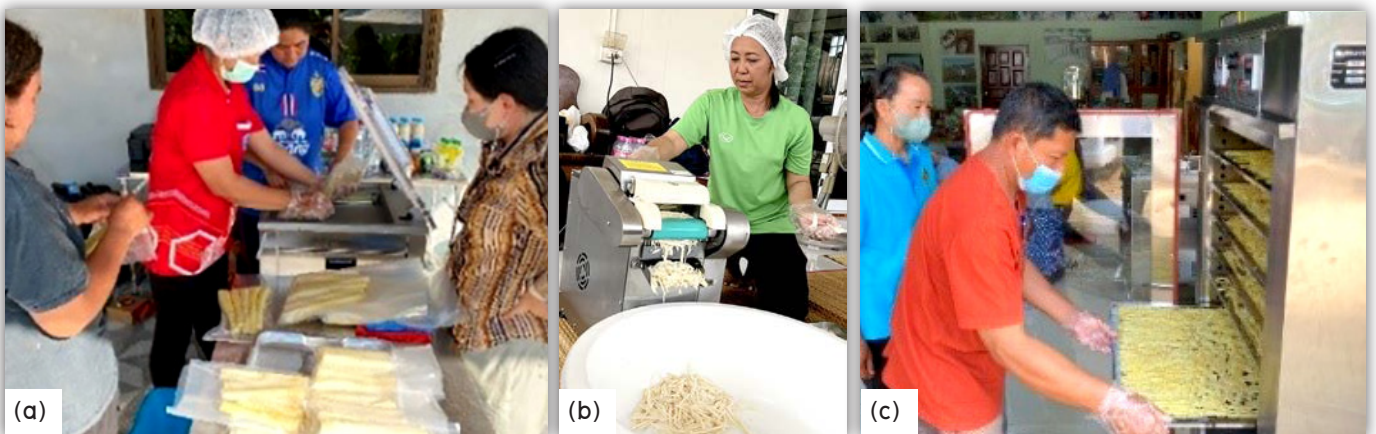
Figure 7 (a) Vacuum packaging kit, (b) Strip and slice bamboo shoot cutting machine, and (c) Temperature adjustable hot air incubator
