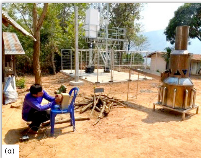
Figure 9 (a) Energy conservation charcoal furnace and (b) Charcoal grinder
