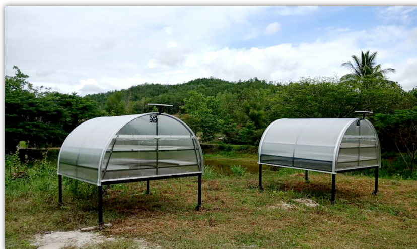
Figure 3 Solar ovens from the department of alternative energy development and efficiency
