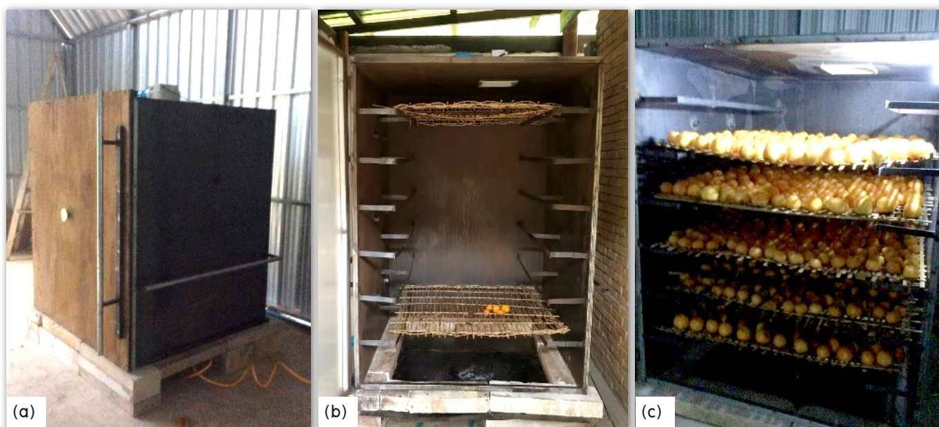
Figure 4 Persimmon processing machine farmer group; (a) Conventional dryer, (b) Inside conventional dryer, and (c) Traditional processed persimmon
