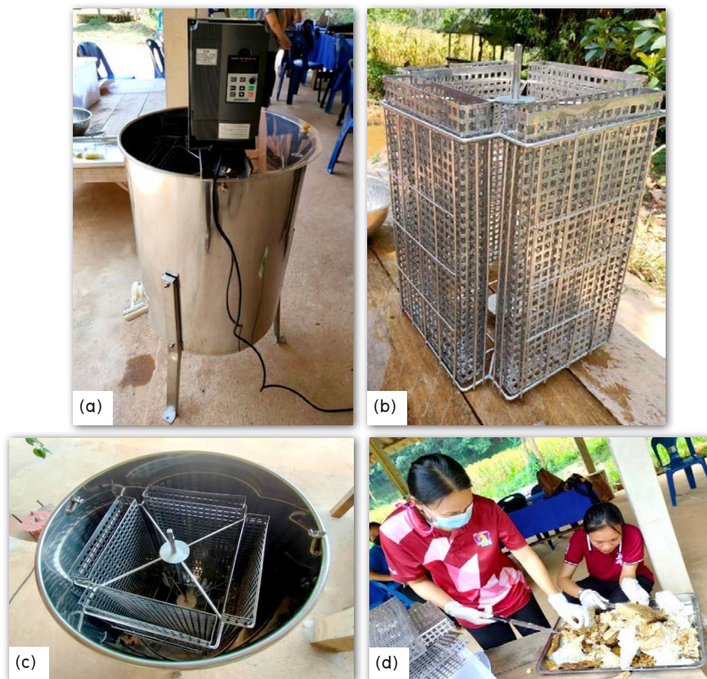
Figure 5 Honey separator for wild bees with inverter speed control; (a) Honey extractor machine, (b) Grating set, (c) Rotating, and (d) Bee hive preparation
