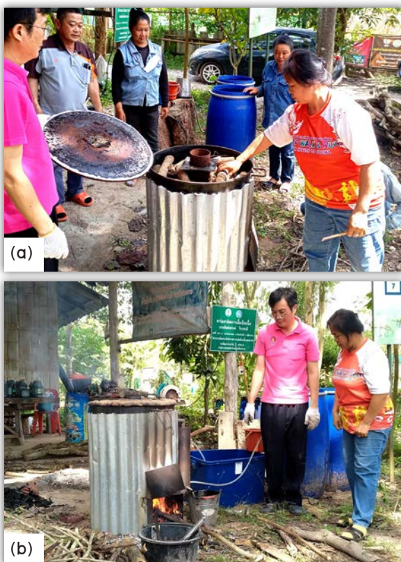
Figure 5 Training the trainers; (a) Training innovators on furnace preparation, (b) Training innovators on burning techniques, and (c) A 200-liter tank charcoal production furnace prototype
