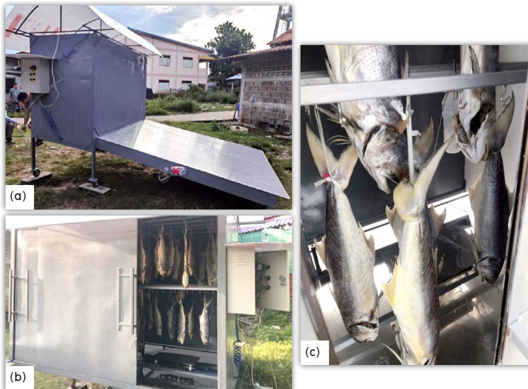
Figure 6 Drying process of salted four-finger threadfin; (a) Full-scale solar dryer, (b) Sliding door for the solar dryer, and (c) Hanging fish inside the drying chamber
