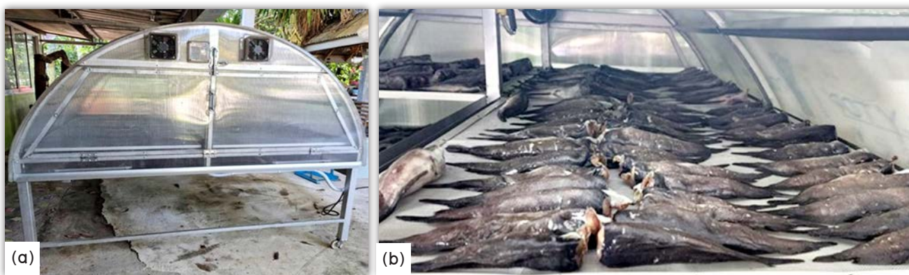
Figure 7 (a) Fish drying cabinet powered by solar energy and electricity and (b) Drying of dry-fermented catfish product
