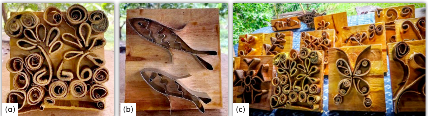
Figure 6 Batik printing blocks made of (a) Blockdried sheath of araca palm compared to (b) Aluminum and (c) Variety of patterns developed during the design process
