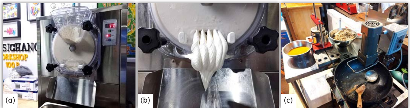
Figure 2 Examples of equipment and materials procured to enhance the production process of blue crab processed ice cream; (a) Batch ice cream freezer, (b) Ice cream extrusion and texture formation process, and (c) Semi-industrial food processing equipment
