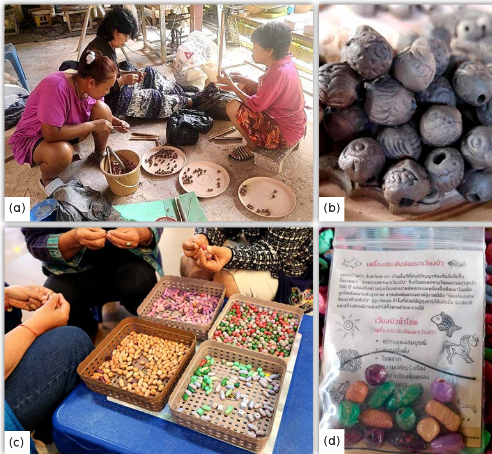
Figure 8 Wiang Bua ceramic bead jewelry co-creation process; (a) Clay forming, (b) Pattern imprinting, (c) Customer workshop, and (d) Final products with packaging
