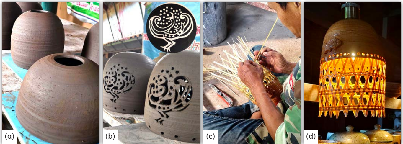
Figure 6 Wiang Bua ceramic lamp design process; (a) Clay forming, (b) Pattern carving, (c) Bamboo integration, and (d) Finished lamp with light effects
