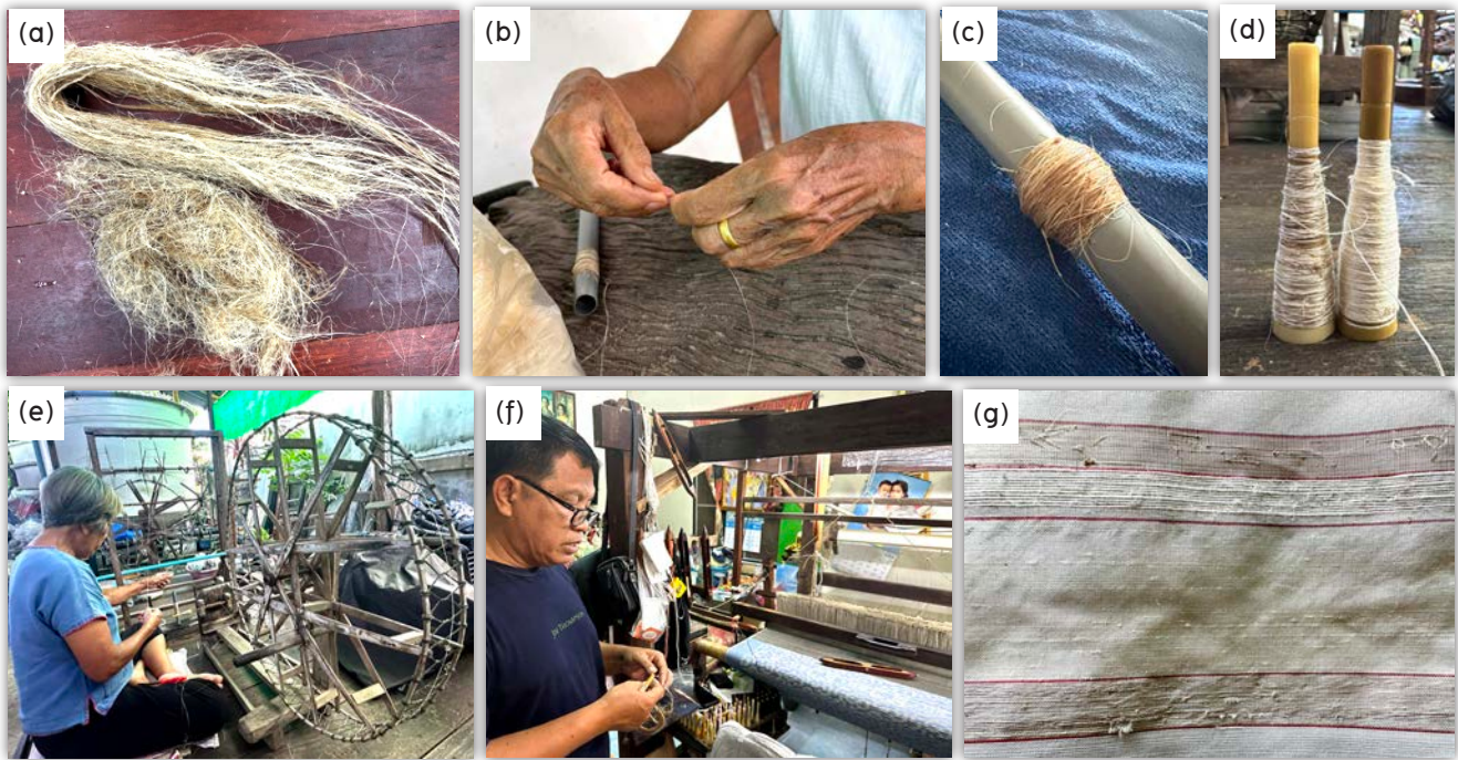
Figure 5 (a) Banana fibers, (b) Splicing fiber, (c) Tensioning the yarn, (d) Winding the yarn onto the bobbin, (e) Yarn doubling, (f) Handweaving, and (g) Banana fiber blend fabric
