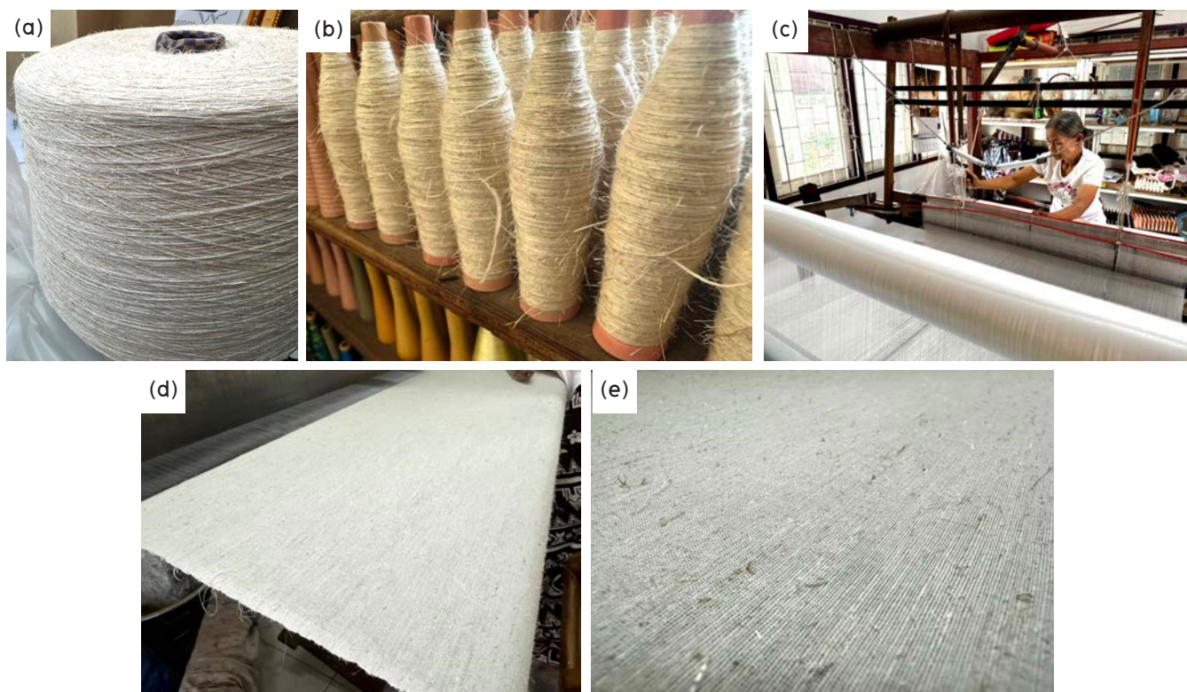
Figure 10 (a) Banana fiber hybrid textile innovation, (b) Shuttle, (c) Handweaver, (d) Handweaving textile, and (e) Handwoven banana fiber blend fabric
