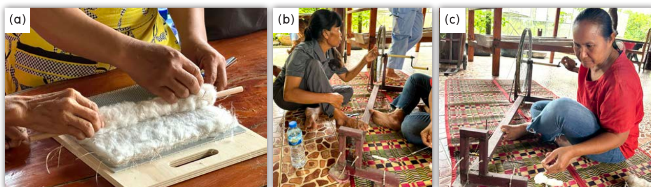
Figure 7 (a) Fiber blending, (b) Fiber spinning, and (c) Handwoven
