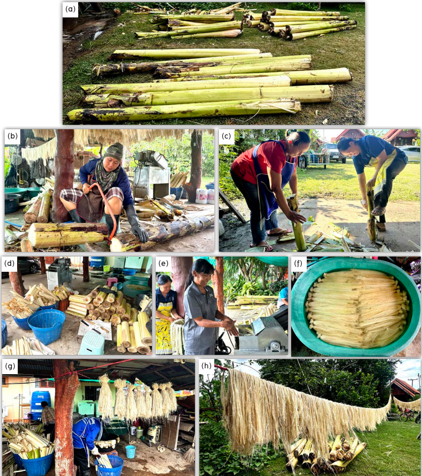
Figure 9 (a) Raw material preparation, (b) Banana pseudostems cut to 60 cm in length, (c) Preparation of banana pseudostems, (d) Raw material preparation, (e) Fiber extraction by machine, (f) Fiber treatment, (g) Shade drying, and (h) Open-air drying
