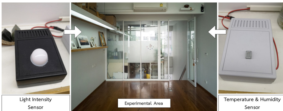
Figure 3 Light intensity sensor (Left) Experimental area (Middle), and temperature and humidity sensor (Right)
