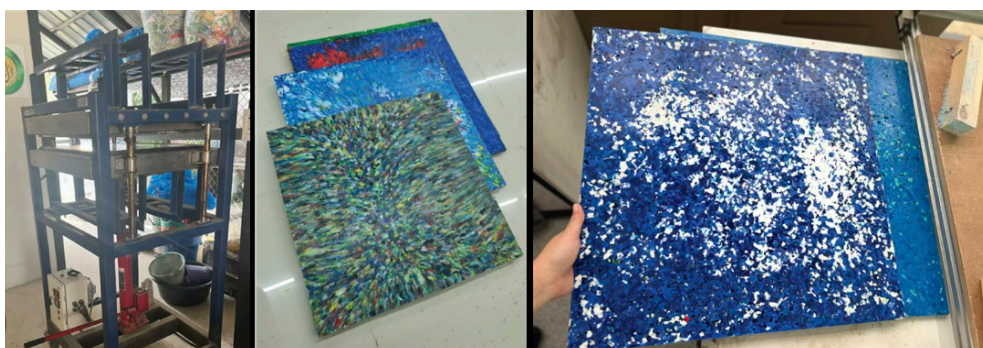
Figure 3. The plastic press machine and the plastic produced from the pressing process
