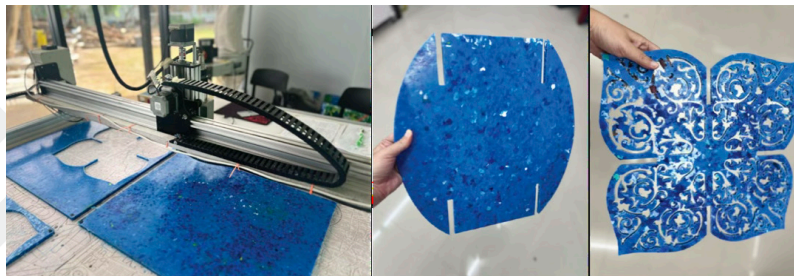
Figure 11. CNC laser cutting of plastic sheets
